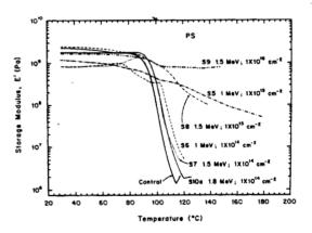
Fig. 7. Pristine PS storage modulus E, compared with the E of samples irradiated at different fluences and energies. S-9 sample is the most crosslinked.
