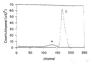
Fig. 4. Spectrum of protons scattered at 30°, showing the C and H peaks, separated by kinematics.
