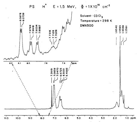
Fig. 1. NMR spectra of PS irradiated with protons of E = 1.5 MeV and  $\Phi = 1 \times 10^{16}$  cm<sup>-2</sup>. For convenience, the region between 7.5 and 8.2 ppm of the spectrum, shown at the left top, has been enlarged.
