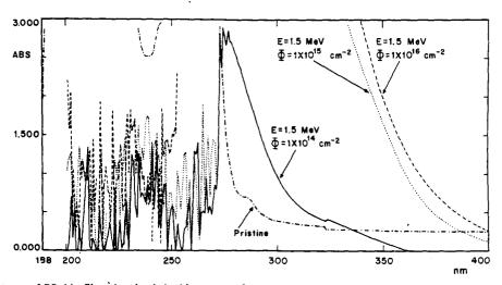
Fig. 2. UV-Vis spectra of PS thin films, bombarded with protons of energy = 1.5 MeV at different fluences. The spectrum of the pristine, which was sub-tracted from each irradiated sample, is also shown.
