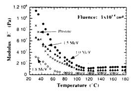
Fig. 12. Plot of the storage modulus E of pristine and irradiated LDPE.
