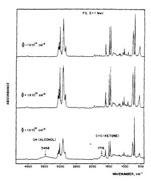
Fig. 1. FTIR spectra of PS irradiated with protons of E = 1.0 MeV and  $\Phi = 1 \times 10^{16}$  cm<sup>-2</sup>, showing new bands at 3468 and 1716 cm<sup>-1</sup>.
