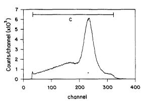
Fig. 3. Spectrum of protons backscattered from C at a laboratory angle of 150°. The shape is due to resonance scattering.
