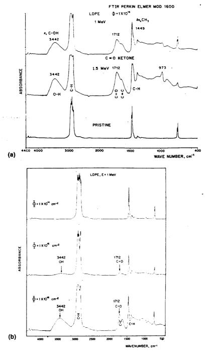
Fig. 9. (a) FTIR spectra of LDPE, control and irradiated with protons of 1.0 MeV at  $\Phi = 1 \times 10^{16}$  cm<sup>-2</sup>, showing new bands as well as an absorption increase in the 1400–700 cm<sup>-1</sup>. (b) FTIR spectra of LDPE, irradiated with protons of 1.0 MeV and three different fluences, the new bands show up the presence of OH and C=O groups.
