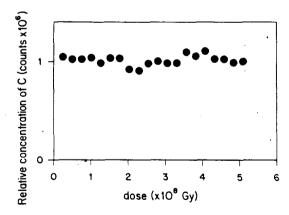
Fig. 5. Variation of the C concentration with dose, obtained from backscattered spectra.
