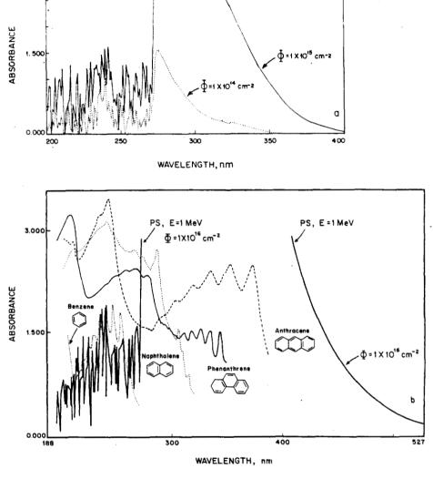
Fig. 2. (a) UV-Vis spectra of PS thin films, bombarded with protons of 1 MeV energy at different fluence. (b) UV-Vis absorption spectra of polycyclic structures (see Ref. [17]). For convenience, Benzene spectrum was slightly shifted. For comparison, S-4 sample spectrum, obtained in this study, is shown in wide solid line.
