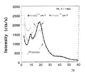
Fig. 5. WAXS diffractograms of PS films, pristine and irradiated with protons of 1.0 MeV at fluence as indicated.
